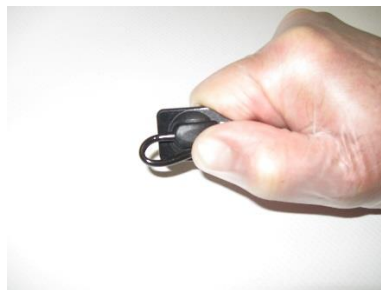
DO NOT pinch sensor or cable
